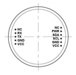
\* Note: Two VCCs are connected internally.
